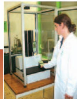
*The STENTOR can be placed in a closed cabinet if sample rupture presents a risk for the operator. In that case, the motor stops as soon as the cabinet door is opened.*
