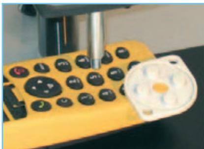
Thanks to its many calculation possibilities, the CENTOR Star force gauge can be used to fully characterize switches, contactors, circuit breakers and keyboards.
